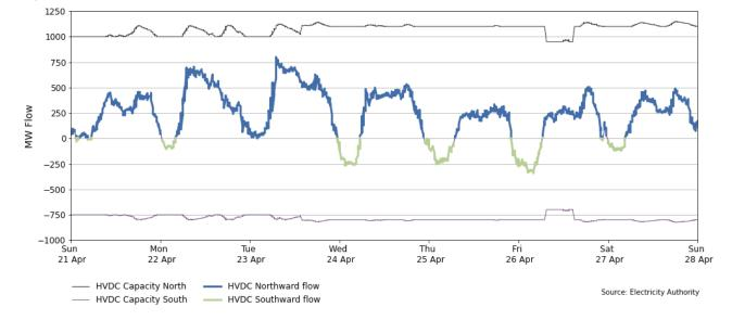
Figure 6: HVDC flow and capacity between 21-27 April
