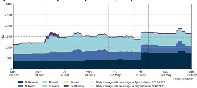
Figure 17: MW loss from thermal outages between 28 April-4 May
