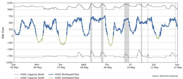
Figure 6: HVDC flow and capacity between 5-11 May
