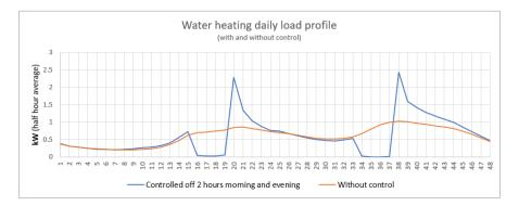
It is very clear to see that managing load and eliminating the diversity can create spikes (the blue line) that are much greater than the load would be if we left it alone (the orange line). Good management of water heating load has the potential to remove 1kW of load per household. Poor load management runs the risk of instead adding 2kW.
