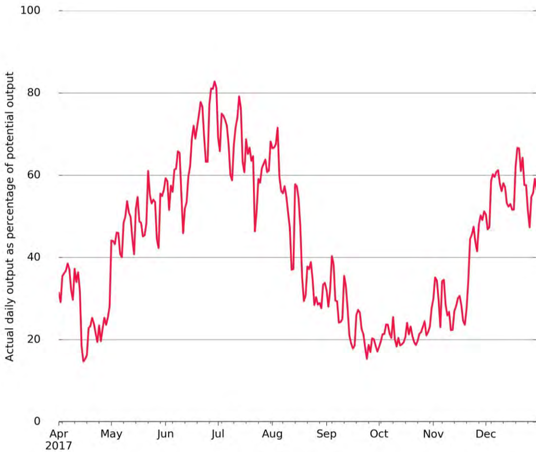
Figure 6: Daily thermal output as a percentage of potential output
